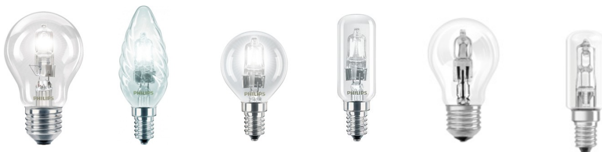
Figure 3a. Non-directional mains voltage halogen lamps class C. Popular type names: 'Eco-classic' (Philips, OSRAM), 'HaloGLS' (GE). Shapes: classic bulb, candle, twisted candle, ball, tubular. Caps: screw-type (E14, E27 as in picture) or bayonet-type. Common power range 18-28-42-53-70-105 W. Rated product life 1500-2000 h (to be restricted to \geq 20000 h after 1.9.2013). Voltage in EU: 220-240 V (hereafter '230 V'). Prevalently used as replacement lamp for incandescent lamps. Declared energy class 'C'. Consumer list prices of A-brands, including tax, up to € 3.5-4 per unit. Street prices of grey-brands, including tax, can be found as low as € 1.5 per unit.
