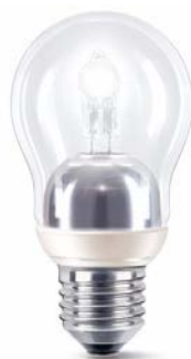
Figure 3b. Non-directional mains voltage halogen lamps class B. This lamp was brought on the market in a 20 and 30 Watt version by Philips in 2008. Philips production stopped in 2010, reportedly for lack of commercial success. The retail price was € 9.95 and declared life time 3000 h. The lamp was fully dimmable. A voltage transformer was incorporated in order to host a class B low voltage halogen lamps (figure 2b). Currently Chinese-made lamps exist with similar design (i.e. with transformer), similar price and –as far as could be assessed– similar lack of commercial success; it could not be ascertained whether these lamps meet the class B requirements.
